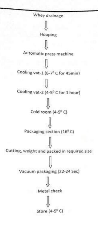
Equipments: Storage tank, Double jacket VAT with agitator, Heat exchanger, Hoops (pressing device), Brine tank, Cold Storage, Weighing machine, Vacuum packaging machine, Deep freezer.
